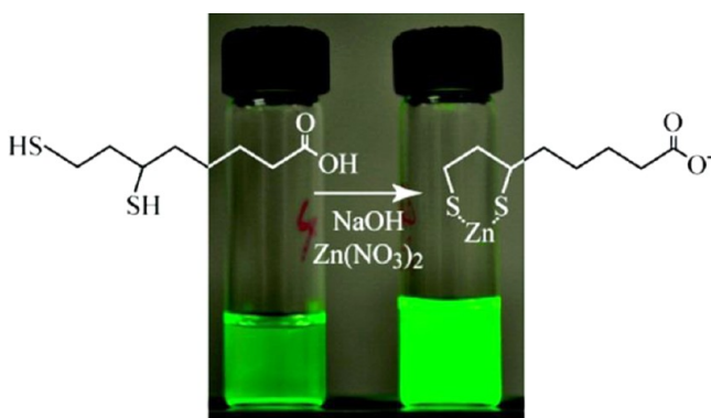
Figure 9. Qualitative photoluminescence of QDs passivated with DHLA (left) and DHLA following a treatment of NaOH and Zn(NO_3)_2 (right). Reprinted with permission from ref 121. Copyright 2010 American Chemical Society.
